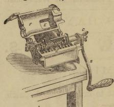
The patented arrangement in this Machine is a longitudinal opening in the side of the Cylinder, fitted with a Sliding Door, so as to allow the meat to pass through cut as fine as butter for Potted Meats; or by enlarging the opening, it can be cut various sizes for Mincing purposes, or coarser for Hashes, Pies, &c. It will cut Vegetables for Soups, also Mash Potatoes, Cut Fruit and Suet.
